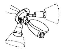
Locate shield slots and push down over four retainer pins.
